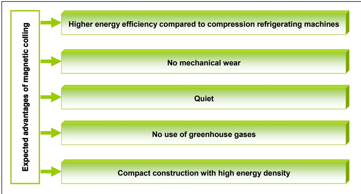
Figure 22 Expected advantages of magnetic cooling
